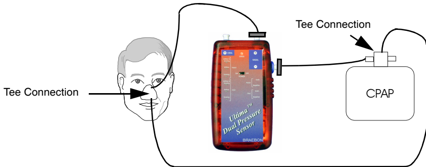
Figure 8 CPAP mask connection and CPAP tee connection to the nasal differential input
