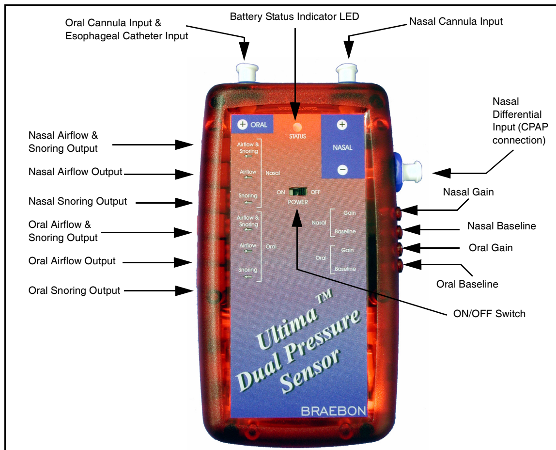
Figure 1 The Ultima Dual Airflow Pressure Sensor™ (Model 0580Pes)
