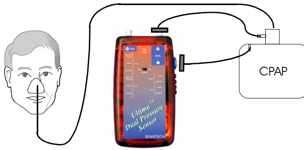
Figure 7 CPAP adapter connection and connection to the nasal differential input
